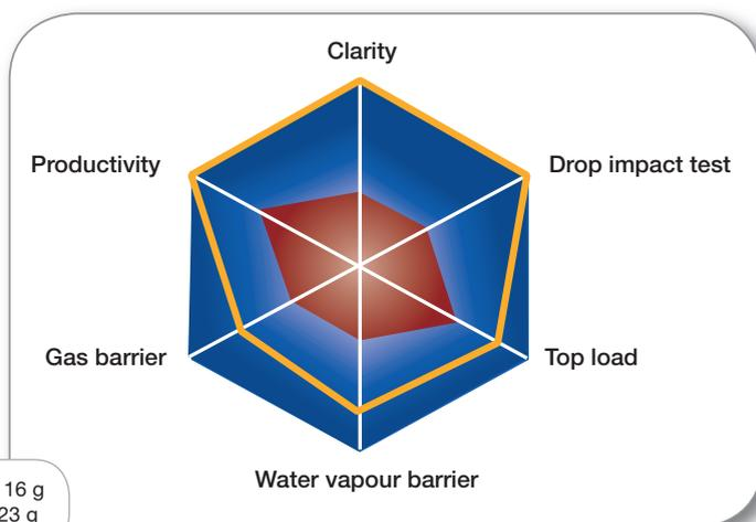
The graph illustrates the advantages of bi-orientation in the case of hollow container production: an Extrusion Blow Moulded bottle is compared to an Injection Stretch Blow Moulded one.
